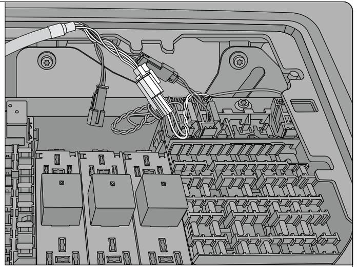
**Step 4:** Remove the terminating resistor and then plug it into the mating end of the HRN-CE10A2.
