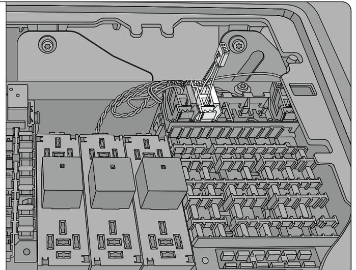
**Step 2:** Connect the 2-pin white connector from the kit into any spare constant power slot. Test for power with a multimeter to verify.
