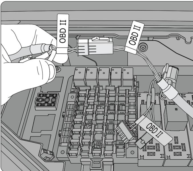
**Note:** Connect the 6-pin white molex connector on white HRN-CE10A2 to the 6-pin white molex connector on the HRN-CM24Y1. They are both labeled OBD2.
