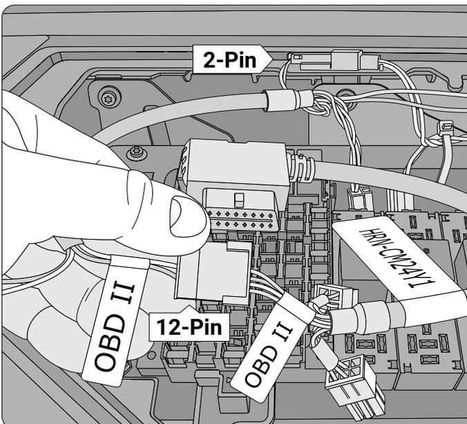
**Note:** For Volvo vehicle models from 2004 to 2007 where the 2-pin gray J1939 connector is not available – Plug the 2-pin black connector of the HRN-CE10A2 (green and brown wires) into the mating 2-pin black connector in the top passenger corner of the fuse box. Next, connect the 12-pin black Molex connector on the HRN-CE10A2 to the corresponding connector on the HRN-CM24Y1. They are both labeled OBDII.
