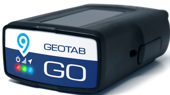
The Geotab device installed in each vehicle collects telematics data for reporting purposes.
